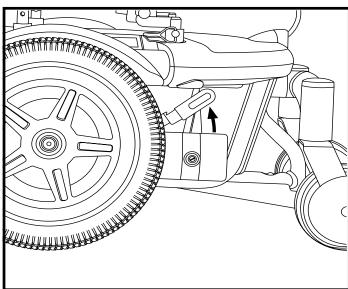
Figure 8. Drive Mode (Drive Engaged)
